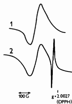
Fig. 8. EPR spectrum of the reaction intermediate in reaction of Rhmnt_2^{2-} with CH_3I . 1: 10^{-3} \text{ mol} \cdot \text{l}^{-1} [Bu_4N]_2^- [Rhmnt_2] ; 2: 315 seconds after addition of 4 \cdot 10^{-4} \text{ mol} \cdot \text{l}^{-1} CH_3I .
